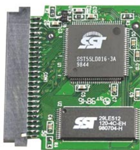
Figure 3. Inside printed circuit board of a CompactFlash (courtesy of Silicon Storage Technology, Inc.).
