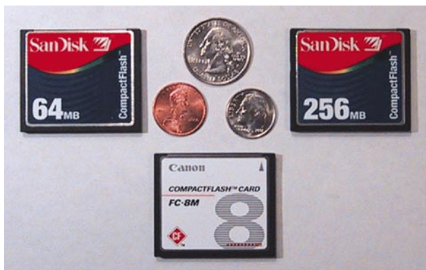
Figure 1. CompactFlash storage card size comparison. CompactFlash and CF are trademarks of the CompactFlash Association.
